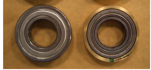
Fig. 2 Original opposite bearing and its replacement
