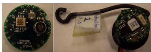
Fig.2 Accelerometer sensor node
