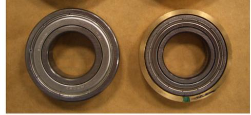
Fig. 2 Original opposite bearing and its replacement
