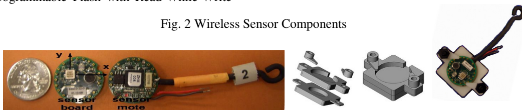
(a) Quarter Size Mica2Dot Sensor Node and Casing
